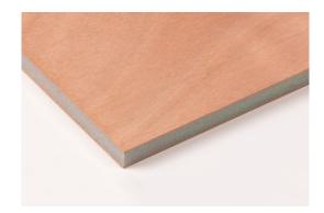
Peeled Okoume Veneers 10/10ths Veneer Quality: II/III Okoume plywood faces with a XPS foam core of various density, from 30 up to 200 kg/m<sup>3</sup>. Standard EN 323.
